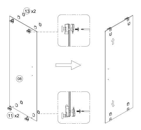
Step A: Locate the rollers into the top and bottom rails.
